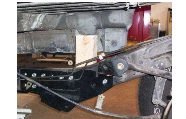
Figure 39 Wood block installed at #4 body mount
