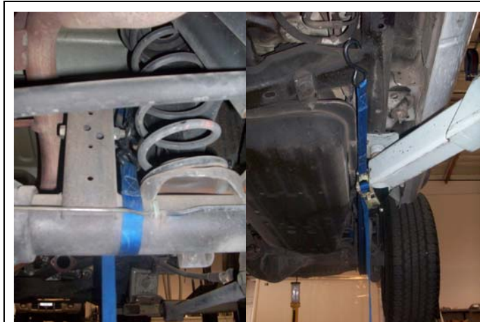
Figure 14 Ratchet strap installed -
