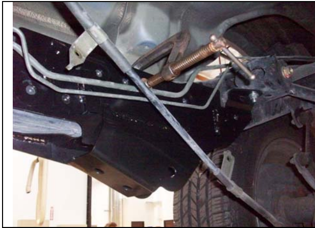
Figure 44 Type "B" bracket temporary installation.
