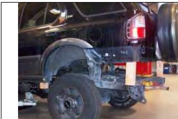
Figure 38 Wood block installed at #5 body mount
