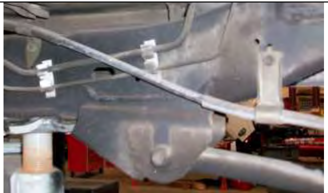
Figure 41 Passenger side bracket before removal
