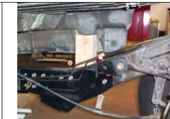
Figure 39 Wood block installed at #4 body mount
