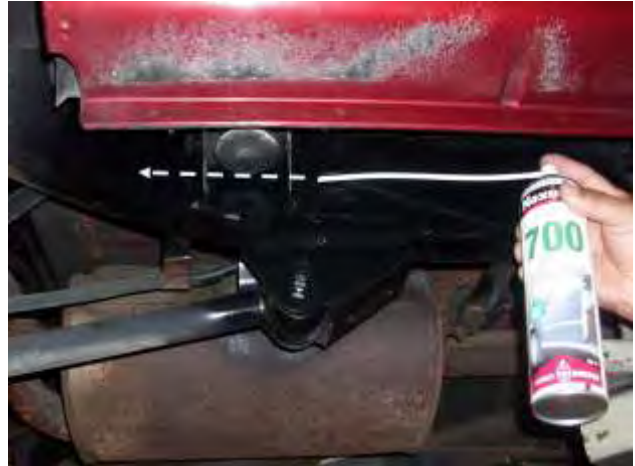
Figure 11 - Frame Hole toward rear 300mm
