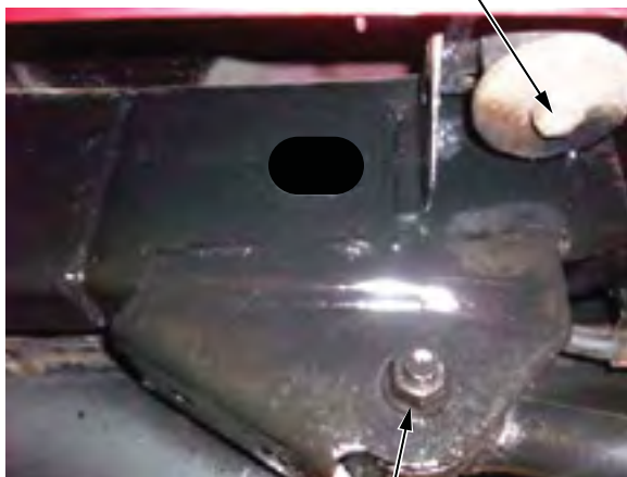
LOWER TRAILING LINK FRONT MOUNTING NUT (Remove.)
