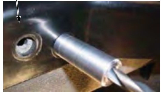
1/4 IN. DRILL GUIDE AND BIT DRILLING THROUGH TYPE B BRACKET AND INTO FRAME
