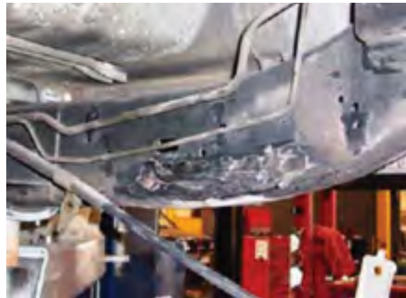
VIEW OF INBOARD FRAME AFTER BRACKET REMOVAL
