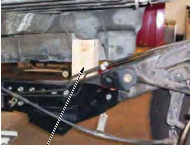
WOOD BLOCK INSTALLED AT #4 BODY MOUNT
