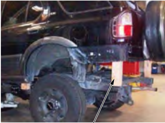
WOOD BLOCK INSTALLED AT #5 BODY MOUNT
