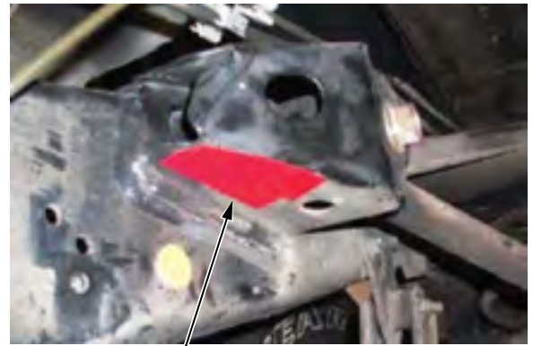
UPPER TRAILING LINK BRACKET COVERED WITH MASKING TAPE
