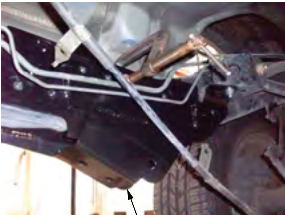
REINFORCEMENT BRACKET (Hold each bracket in place with a new body mount stud and bolt, and a C-clamp.)
