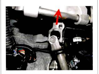
7. Insert the steering column-to-U joint bolt into the bolt hole and check that the bolt passes through the groove.
