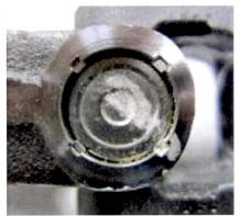
3. Visually check that the steering pinion splined shaft and the U joint are properly connected as shown in the picture on the right.
