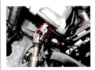
Inspect the bolt for damage/ stripping/cross-threading. Inspect the corresponding threads in the U-joint. Replace both if damage is found.
