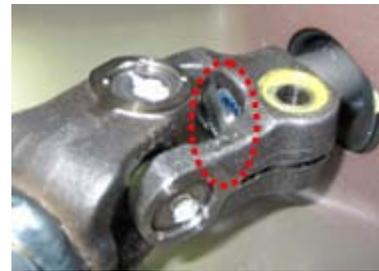
6. Inspect the bolt for damage/ stripping/cross-threading. Inspect the corresponding threads in the U-joint. Replace both if damage is found.
