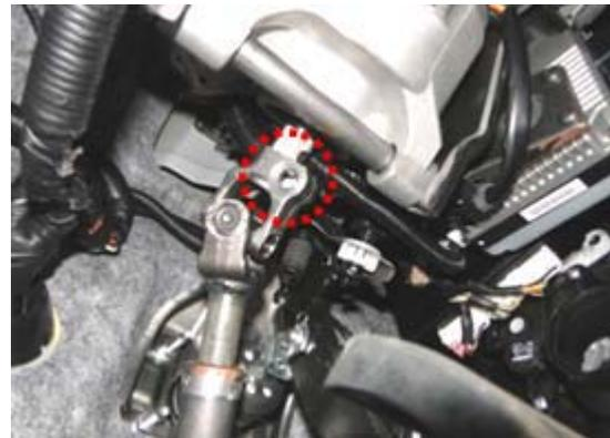
5. Inspect the bolt for damage/ stripping/cross-threading. Inspect the corresponding threads in the U-joint. Replace both if damage is found.
