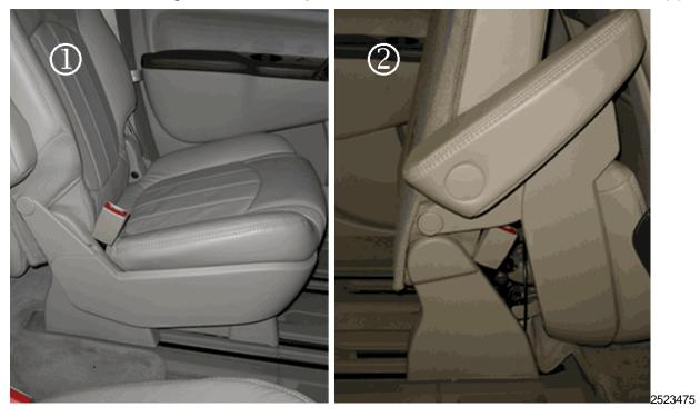
(1) Left hand bucket seat in its normal seating position. (2) Left hand bucket seat in smart slide position. This is the position that the seat must be in to remove the recliner inner trim cover.
