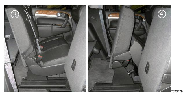
(3) Left hand 60 percent bench seat in its normal seating position. (4) Left hand 60 percent bench seat in the smart slide position. This is the position that the seat must be in to remove the recliner inner trim cover.
