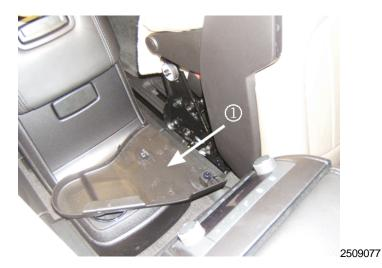
4. Remove the rear seat recliner inner trim cover (1). Refer to Rear Seat Recliner Outer Finish Cover Replacement - Inboard in SI.
