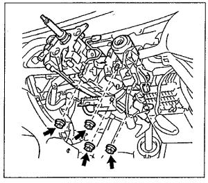
b) Reinstall the steering column assembly with the 4 nuts and torque to spec.
