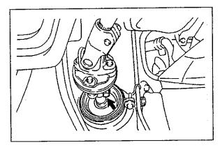
Reinstall the bolt to the intermediate shaft sub-assembly and torque to spec.
