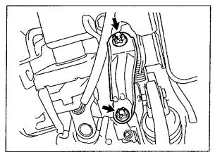
e) Reinstall the pedal bracket stay No. 1 with the 2 nuts and torque to spec.
