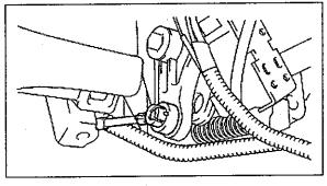
b) Reconnect the transmission control cable to the shift lever housing.
