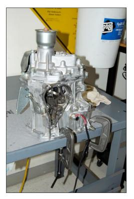
14) Before installing the jig to the transfer case, ensure that the drill bit moves freely within the guide. If the drill bit catches the bracket on the backside of the jig, lightly tap the bracket to allow free movement of the drill bit.
