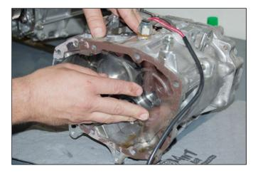
13) Use the included C-clamps to secure the transfer case to a workbench.
