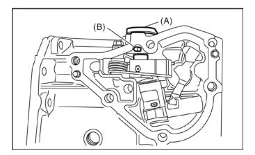
10) Set and hold the selector lever to the 1st-2nd side, and remove the transfer case and extension case assembly as a unit.
