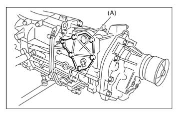
Note: Remove straight pin (B) and set aside. Selector Lever (A) will remain in place Caution: Do not drop straight pin into transmission.
