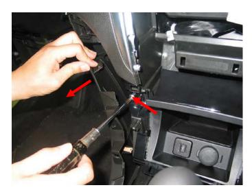
22. While pulling the left side floor console front panel outward, pull the circled part of the instrument panel center lower box backward toward you.
