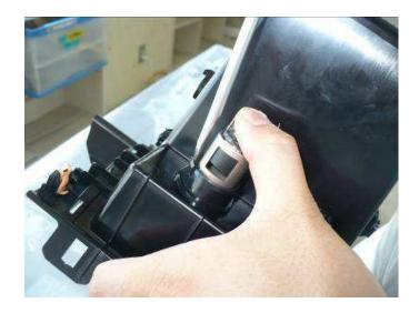
NOTE: Do not apply excessive force to the screwdriver holding the claw to avoid damage to the accessory socket outer cover.
