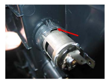
26. To unlock the claw turn the blade of the screwdriver, lifting the claw outward just enough to clear the socket, then push the socket out of the collar.
