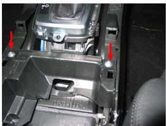
21. While pulling the floor console front panel outward, remove the screw from the center lower box, one each behind the left and right panels.
