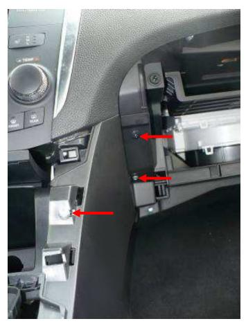
18. With the door of the center lower box open, insert hands behind the lower edge of the HVAC panel and pull outward to remove it.
