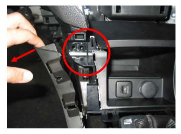
23. While pulling the right side floor console front panel outward, place your fingers under the right lower edge of the box as shown, then lift the center lower box out, exposing the socket connectors.
