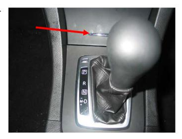
8. Lifting up the front edge of the console rear panel, lift up the rear edge of the black gearshift garnish.
