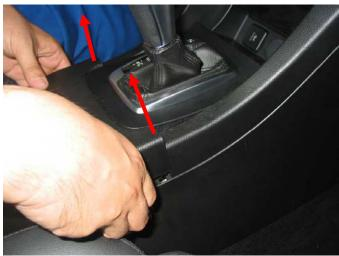
9. There are seven (7) retaining claws that secure the gearshift garnish. These are disengaged in four stages beginning at the rear and moving forward. To disengage the front two points, apply pressure on the garnish pulling slightly back while lifting.
