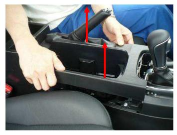
12. Remove the left and right front floor console garnishes by lifting slightly at the rear edge then pulling them backward.
