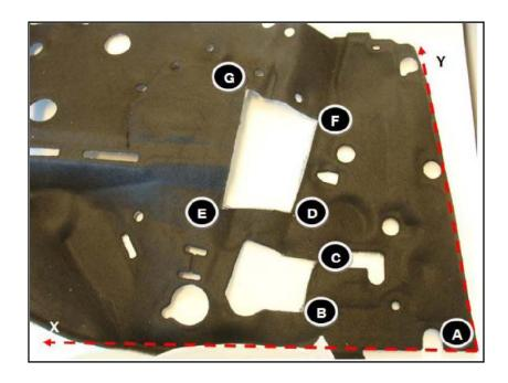
7. Reinstall the modified sound insulation on the left and right quarter panels.
