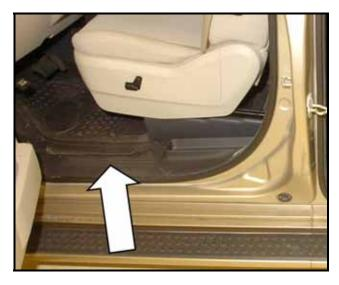
← Reinstall front door sill plate -arrow-
