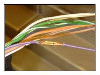
Note: Wires should overlap each other within the band splice as shown; not butt end-to-end
