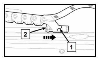
← Lock chain link -1- in place by pushing the locking tab -2- rearward -in direction of arrow-
