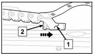
Lock chain link -1- in place by pushing locking tab -2- rearward -in direction of arrow-
