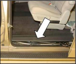
← Reinstall sliding door sill plate -arrow-
