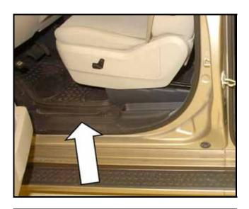
Using trim removal wedge RMCP101 or equivalent, gently pull up on inside edge of the sill plate to disengage clips from body and remove front door sill plate -arrow- from vehicle
