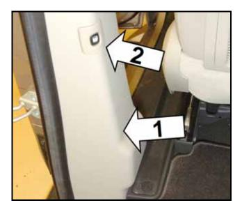
Using trim removal wedge RMCP101 or equivalent, gently remove lower B-pillar trim arrow 1- and disconnect the power sliding door switch -arrow 2- from the body wiring harness connector and remove lower B-pillar trim from vehicle
