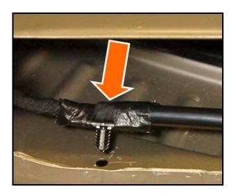
Reposition wiring harness retainer at end of split tube -arrow- and tape wiring harness retainer properly in place with electrical tape
