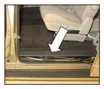
Using trim removal wedge RMCP101 or equivalent, gently pull up on inside edge of sliding door sill plate -arrow- to disengage clips from body and remove sliding door sill plate from vehicle
