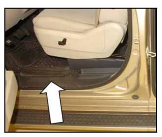
← Reinstall front door sill plate -arrow-
