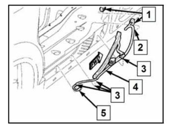
Connect new wiring harness to the second row seating side impact sensor electrical connector -5-
