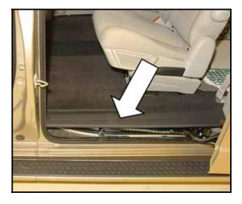
← Reinstall sliding door sill plate -arrow-
