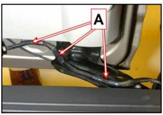
Insert power sliding door wiring harness retainers into lower hinge and sliding door retention holes at positions -A-
