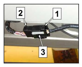
Connect 10-pin power sliding door wiring harness connector -1- into sliding door wiring harness connector -2- and slide gray locking tab -3downward (upward on passenger side)
