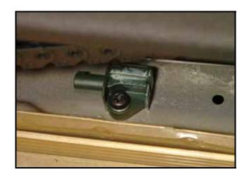
Move power sliding door wiring harness and chain link track forward to gain access to second row seating side impact sensor and disconnect electrical connector, as shown
