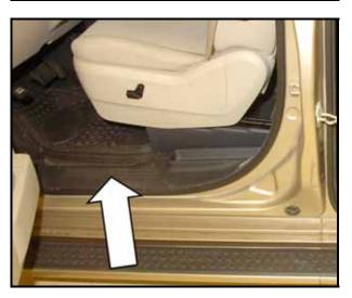
← Reinstall front door sill plate -arrow-
