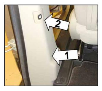
Using trim removal wedge RMCP101 or equivalent, gently remove lower B-pillar trim arrow 1- and disconnect the power sliding door switch -arrow 2- from the body wiring harness connector and remove lower B-pillar trim from vehicle
