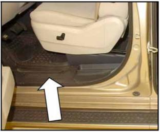
Using trim removal wedge RMCP101 equivalent, gently pull up on inside edge of sill plate to disengage clips from body and remove front door sill plate -arrow- from vehicle
