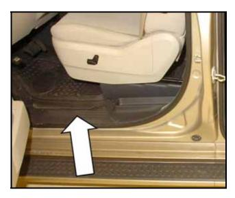
← Reinstall front door sill plate -arrow-
