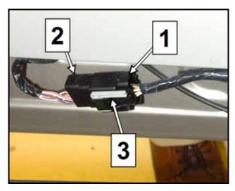
□ Disconnect 10-pin power sliding door wiring harness connector -1- from sliding door wiring harness connector -2- by first pushing the gray locking tab -3- upward (downward on the passenger side) and pushing down on the release tab while separating the connector
