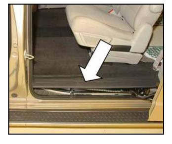
← Reinstall sliding door sill plate -arrow-
