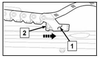
Lock chain link -1- in place by pushing locking tab
