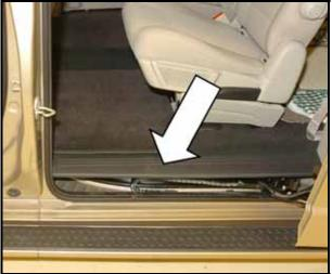
$\leftarrow$  Reinstall sliding door sill plate -arrow-
