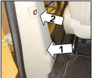
Using trim removal wedge RMCP101 or equivalent, gently remove lower B-pillar trim -arrow 1- and disconnect power sliding door switch -arrow 2- from body wiring harness connector and remove lower B-pillar trim from vehicle
