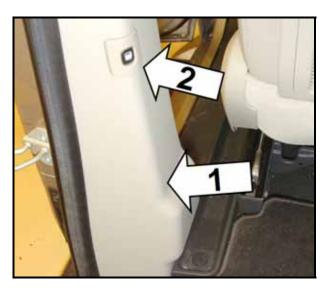
Reconnect power sliding door switch -arrow 2- to body wiring harness connector and reinstall lower B-pillar trim -arrow 1-
