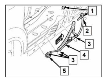
Disconnect 10-pin power sliding door harness connector -1- from body harness connector at the lower B-pillar
