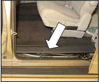
Using trim removal wedge RMCP101 or equivalent, gently pull up on inside edge of the sliding door sill plate -arrow- to disengage clips from body and remove sliding door sill plate from vehicle
