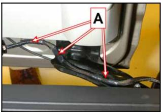
Using Pry Lever tool 80-200 or equivalent, remove sliding door wiring harness from sliding door and lower hinge bracket by carefully pulling wiring harness retainers out of the retention holes -A-
