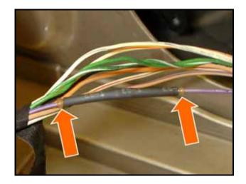
← Center shrink tube over repaired area and use UTI-100SI Ultratorch or equivalent to heat shrink tube until it shrinks around the wire and glue -arrows- protrudes from both ends of the shrink tube, as shown
