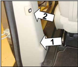
Reconnect power sliding door switch -arrow 2- to body wiring harness connector and reinstall lower B-pillar trim -arrow 1-
