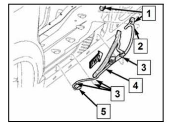
Connect new wiring harness to the second row seating side impact sensor electrical connector -5-
