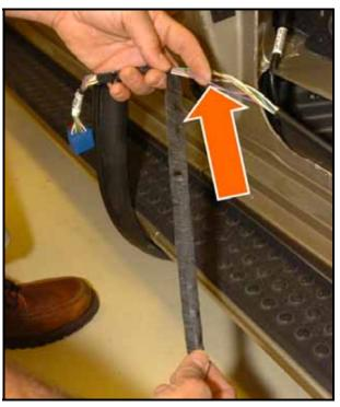
Carefully unwrap power sliding door wiring harness, as shown, starting at the front end (in-car position) of the black plastic split tube to expose chaffed wires -arrow-
