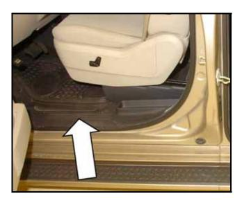
Using trim removal wedge RMCP101 or equivalent, gently pull up on inside edge of the sill plate to disengage clips from body and remove front door sill plate -arrow- from vehicle
