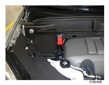
**Note:** The underhood bussed electrical center (UBEC) is located in the engine compartment on the passenger side of the vehicle. Refer to Underhood Fuse Block in the Owner's Manual for fuse information.
