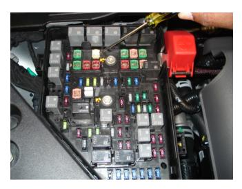
3. Remove the UBEC cover and locate the 60 amp heated windshield washer fuse.
