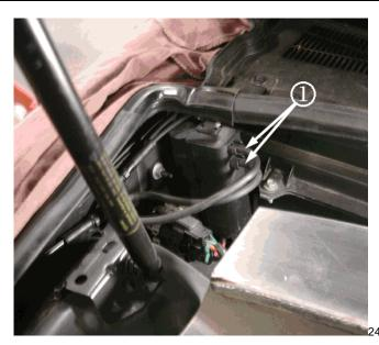
Disconnect the windshield wiper solvent inlet and outlet hoses (1) from the windshield washer solvent heater assembly and from the two plastic inlet and outlet windshield wiper solvent hoses.
