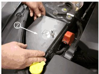
**Note:** The underhood fuse block is located in the engine compartment on the passenger side of the vehicle. Refer to *Underhood Fuse Block* in the Owner's Manual for fuse information.
