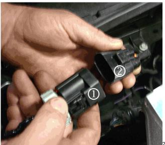
11. Connect the large two-wire connector (1) to the body harness (2).
