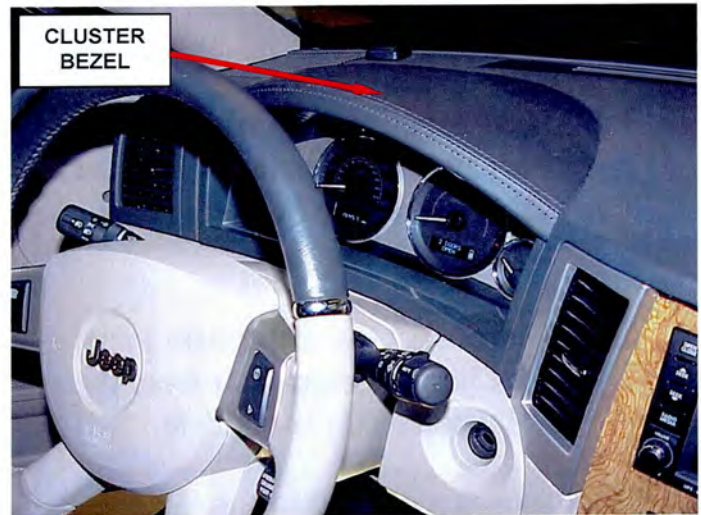
Figure 6 – Cluster Bezel Removal
