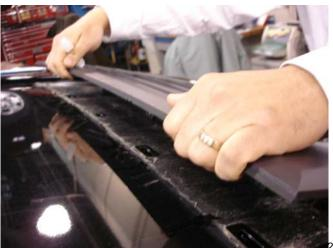
1.2 Continue pulling upward on the hood air grille panel, separating the panel from the hood. Separate the hood air grille panel from the hood beginning on the driver's side corner of the hood air grille panel and finishing on the passenger's side corner of the hood air grille panel.
