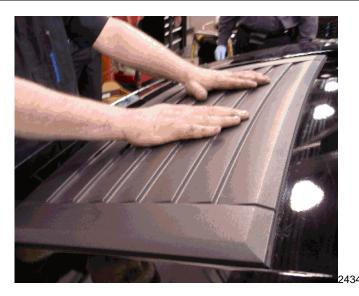
28.3 Apply firm and even pressure over the surface of the hood air grille panel.
