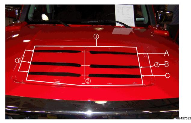
Caution: Dow BetaPrime 5404A or 5404 primer will permanently etch the paint surface of the hood. DO NOT apply primer outside the work area of the hood. Use the top and bottom hood air grille retainer clip slots as the work area border. If primer is accidently applied to paint outside of the work area, IMMEDIATELY clean the area with a shop towel and cleaning solvent such as isopropyl rubbing alcohol 99 percent.
