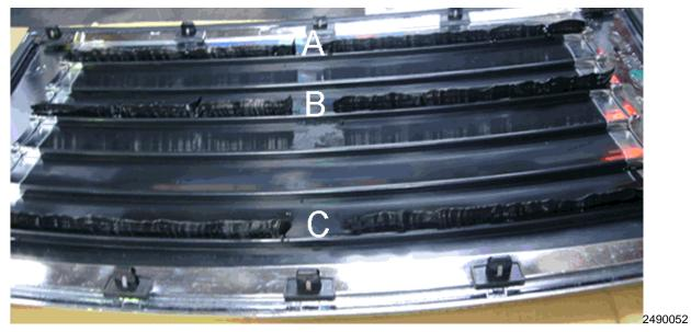
24. Apply Dow Urethane Adhesive U-418 (or equivalent glass-bonding urethane adhesive) to locations (A), (B), and (C) of the hood air grille panel. Six beads of urethane are required.
