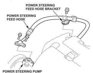
9. Remove the two bolts from the end of the P/S feed hose, then remove the hose from the power steering pump.
