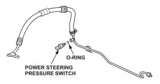
14. Install the new power steering feed hose in the reverse order of removal.
