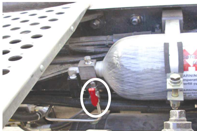
Figure 2. Location of Accumulator shut-off valve, shown in the OPEN (flowing) position.
