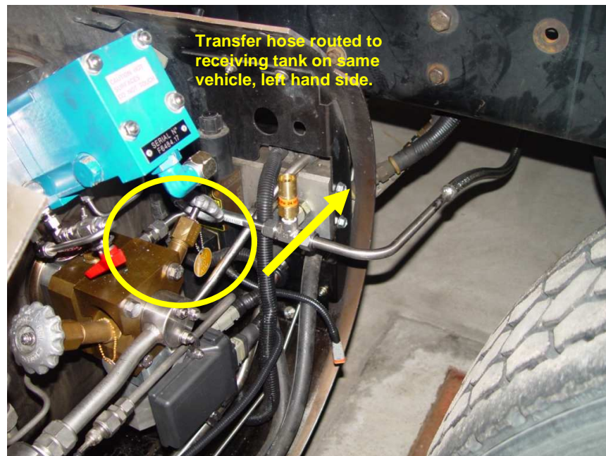
Figure 5. Attachment of the Flexible Transfer Hose, with the hose routed to the receiving tank on the same vehicle, right hand side.
