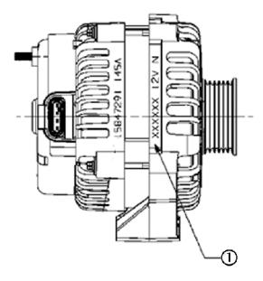
Generator Build Date Location is at the 11 o'clock position on gasoline engines and at the 2 o'clock position for diesel engines. (1) Gasoline Engine Generator Build Date Location shown.
