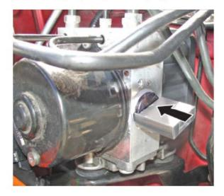
13. Carefully tilt the installer down at an angle to remove it from the cap.
