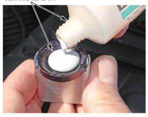
Center the sealing cap installer over the front plug on the VSA Modulator-control unit, and quickly press the cap squarely onto the plug.
