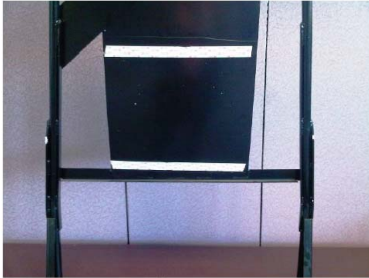
Picture 2 – Adhesive Strip Placement
