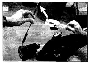
17. Apply the foam tape (L) to the latch assembly starting at the edge of the support bracket and along the side of the latch assembly.
