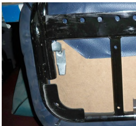
Figure 2: Quarter turn bracket – seat underneath view
