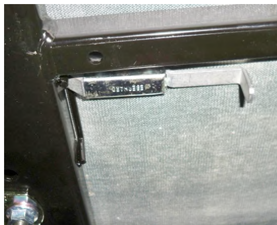
Figure 3: Self latching device – seat underneath view
