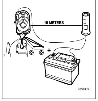
9 Disconnect the detonation device wires from the battery imm ediately after the belt tensioner has been deployed.
