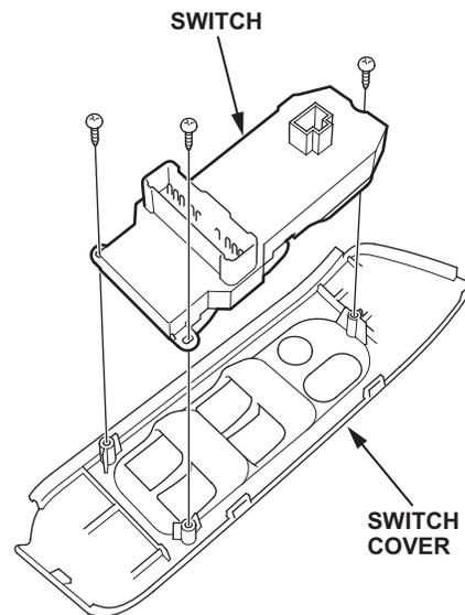
6. Check for corrosion or melting on the switch side and the harness side of the 3P and 20P connectors:
