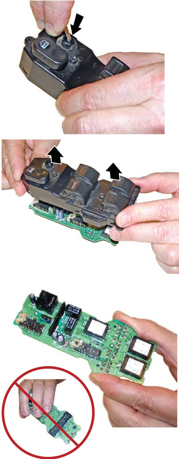
10. Holding the PCB by its edges, check the top and bottom surfaces for moisture damage or corrosion. NOTE: The moisture damage or corrosion can be on any part of the PCB.
