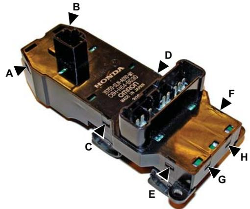
9. Remove the lower half of the switch case, then remove the printed circuit board (PCB) from the top half of the switch case by pushing the main switch area with a flat-tip screwdriver.
