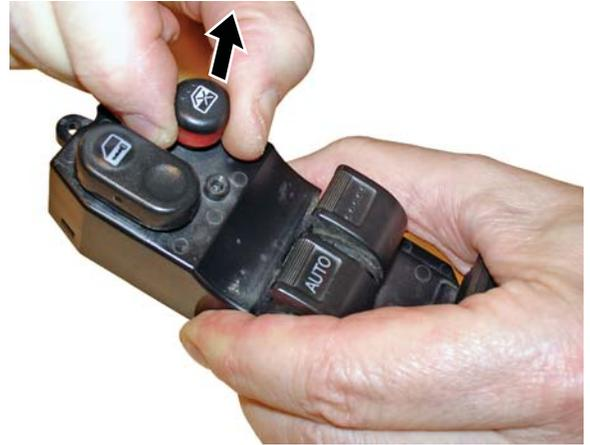
8. Using a small, flat-tip screwdriver, separate the two halves of the switch case:
