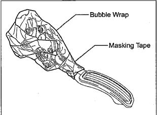
h) While still inside the vehicle, use bubble wrap and masking tape to cover and protect the sensor.
