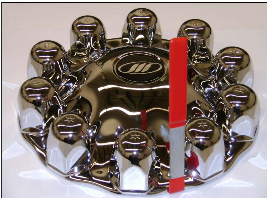
Figure 1. Front / tag axle one–piece hub cover with removal tool.
