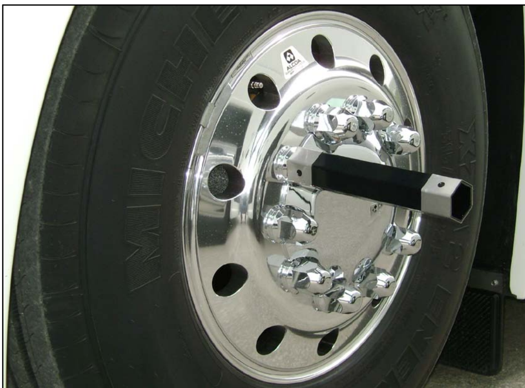
Figure 2. Front / tag axle 11–piece hub cover with removal tool.
