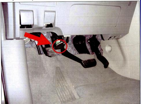
3. Visually inspect the stop light switch bracket shape.
