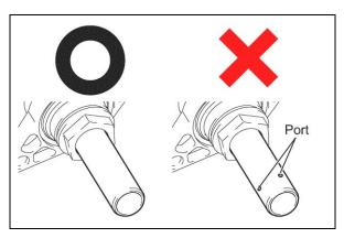
e) Confirm that the piston ports are in the correct position as shown.
