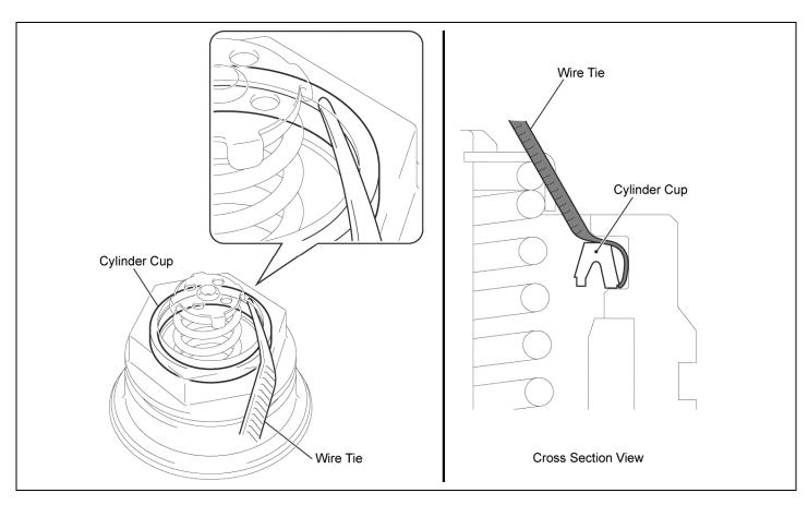
c) Insert the tip of the wire tie over the outside of the Rubber Seal (Brake Master Cylinder Cup) as shown above.
