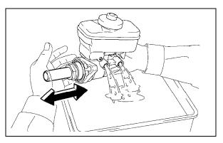
e) Discharge the brake fluid inside master cylinder by slowly moving the piston in and out for 2 complete strokes.
