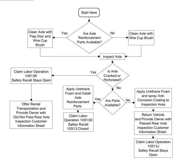
Certain 1998-2003 Model Year Windstar Vehicles Operated in Corrosion States Rear Axle Inspection and Repair
