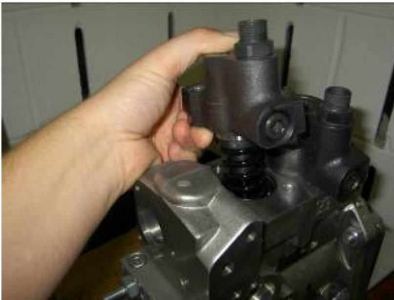
Figure 11 – New Spring And Pumping Element Installation
