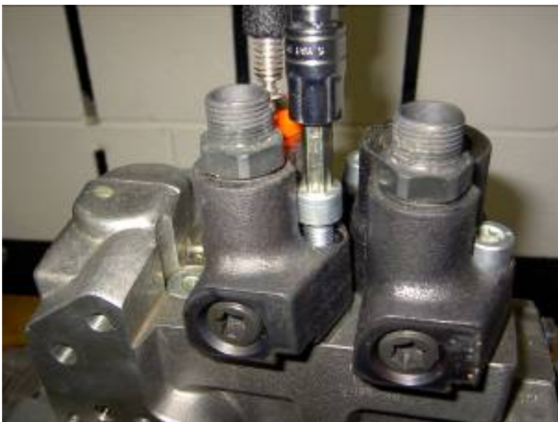
Figure 6 – High Pressure Fuel Pump T-50 Torx Bolt Removal
