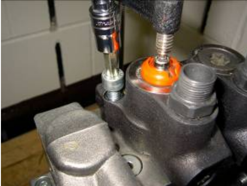
Figure 13 – High Pressure Fuel Pump Element Installation
