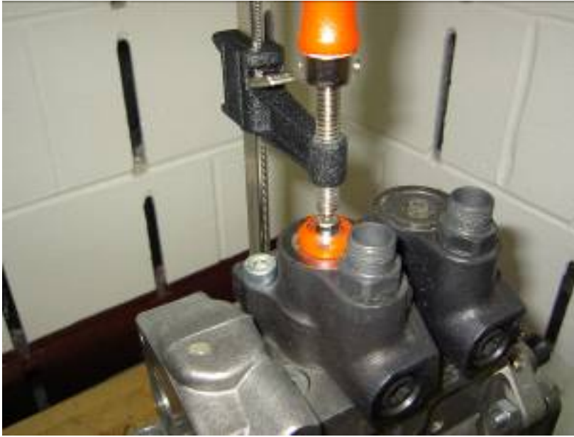
Figure 5 – High Pressure Fuel Pump With C-Clamp On Front Element
