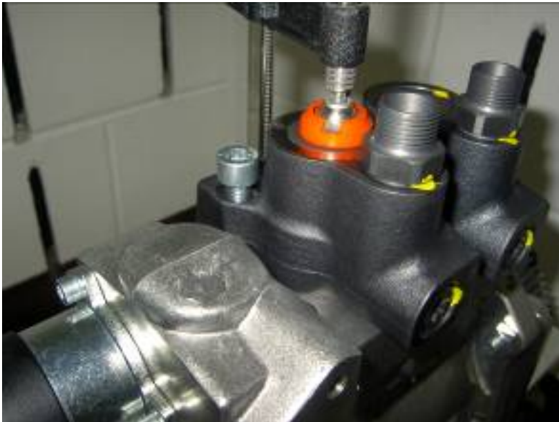
Figure 12 – High Pressure Fuel Pump Element Installation
