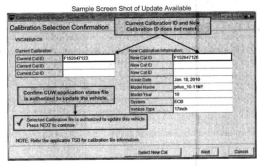
6. If Current Calibration ID from the vehicle does not match the New Calibration ID and the CUW application states "Selected Calibration file is authorized to update this vehicle", then proceed with the update.
