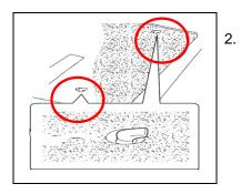
Make sure the floor mat is properly secured by the retaining hooks (clips). Confirm that the retaining hooks (clips) are secured into the grommet holes in the vehicle's floor (carpet).
