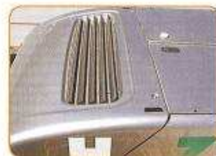
Van Hool craftsmanship visible in the detailed bodywork of the coach, such as these ventilation louvers at the front of the bus.
