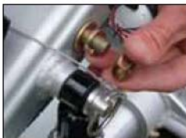
7D Flat washer, lock washer, nut
