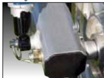
7E Tighten to 57 ft. lbs. (77N-m), right Wheel Block shown
