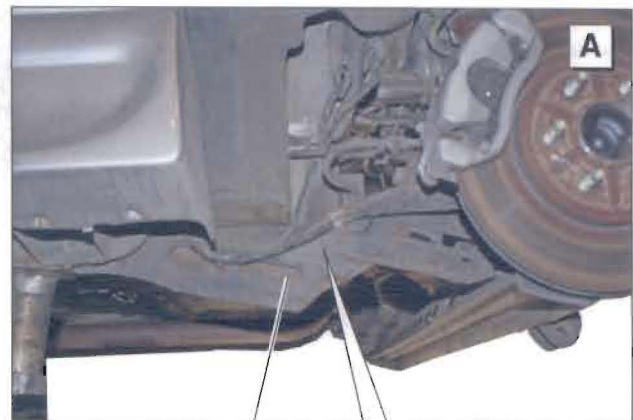
Trailing Arm Inspect this Weld
