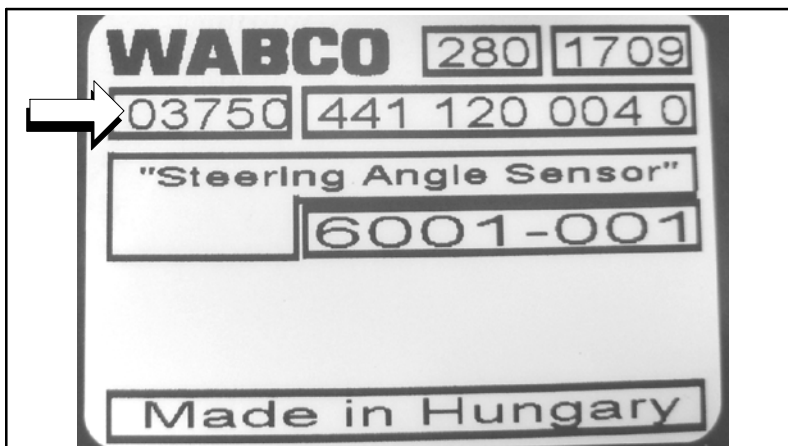
Figure 5. Meritor WABCO steering angle sensor NOT affected by campaign.
