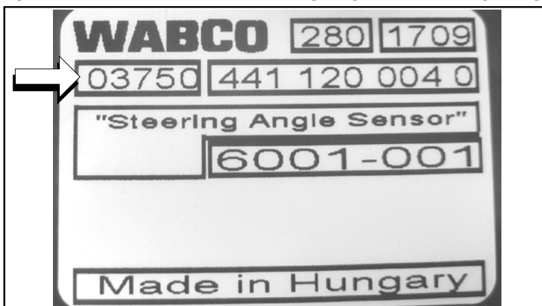
Figure 6. Meritor WABCO steering angle sensor NOT affected by campaign.
