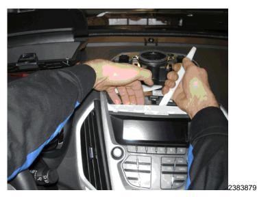
Caution: Insert a plastic body trim tool between the IP and radio control assembly along the top portion of the radio control assembly as shown in the illustration. DO NOT use a flat-blade screw driver to remove the radio control assembly.
