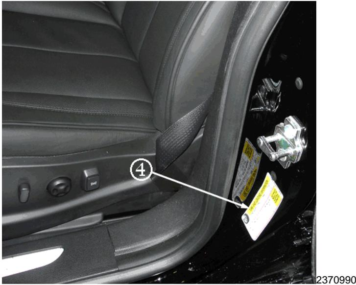
23. Located the B-pillar and affix the provided Tire and Loading Information Label (4) onto the B-pillar as shown in the illustration.
