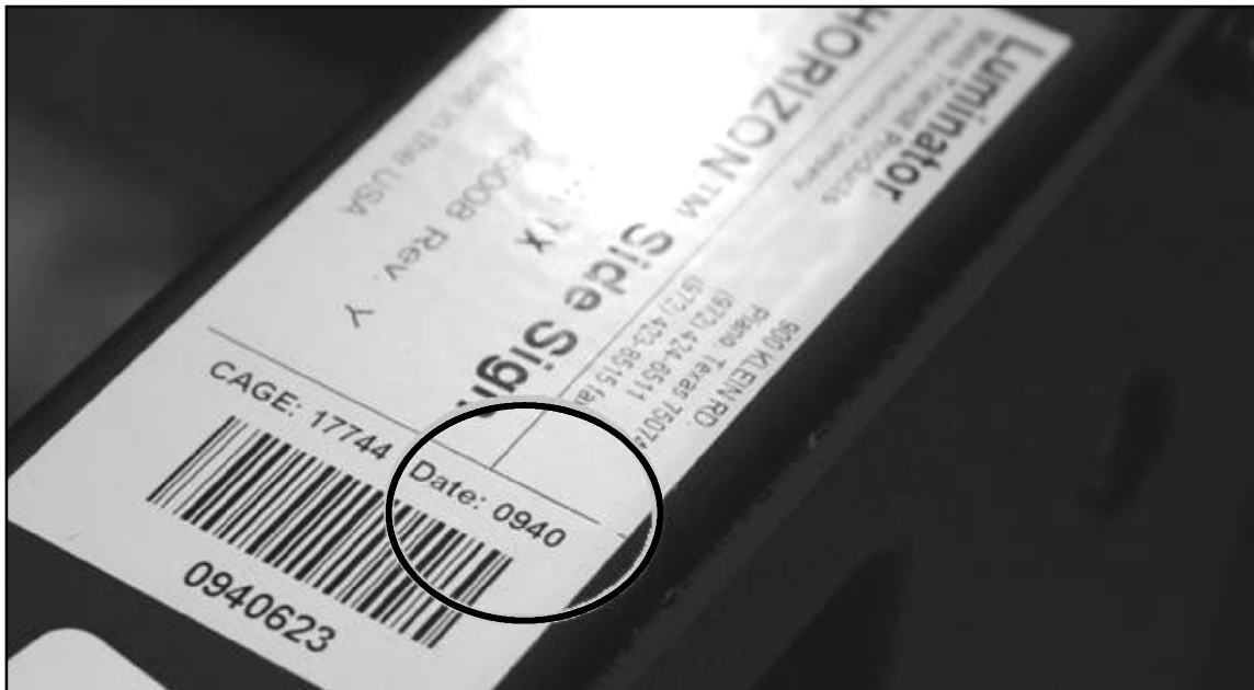
Figure 1. Reference photo of date code product label located on top of the side sign frame.
