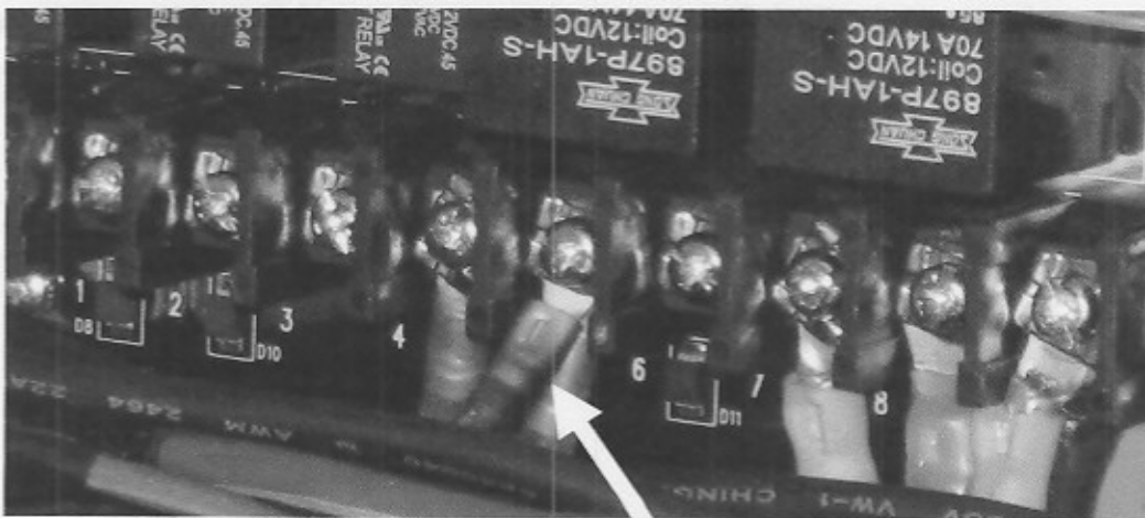
Heat discoloration of a poor (loose) crimp
