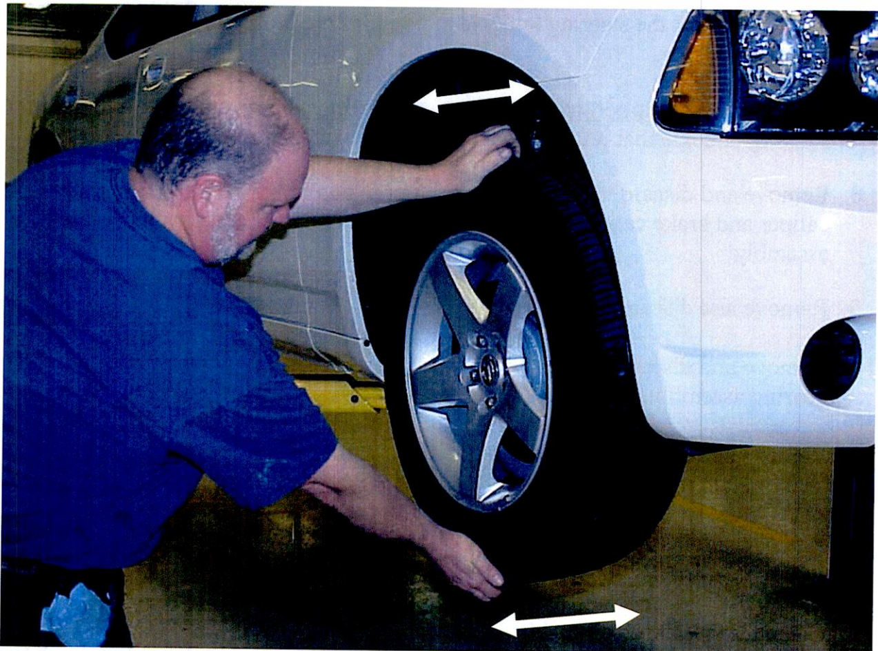
Figure 1 – Check Front Wheels for Looseness
