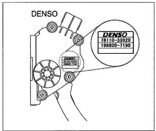
1. IDENTIFY AND REMOVE THE DENSO ACCELERATOR PEDAL ASSEMBLY
