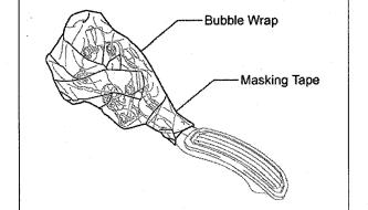
h) While still inside the vehicle, use bubble wrap and masking tape to cover and protect the sensor.
