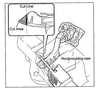
c) Using a reciprocating-saw and cut off the lower section of the pedal as illustrated.
