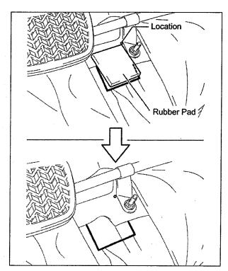
1. Temporarily place the rubber pad on the floor panel as shown, and outline the pad on the sound deadening material with a ball point pen.
