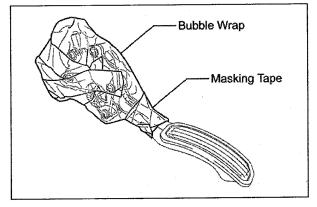
h) While still inside the vehicle, use bubble wrap and masking tape to cover and protect the sensor.
