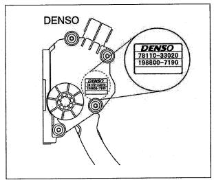
4. IDENTIFY AND REMOVE THE DENSO ACCELERATOR PEDAL ASSEMBLY
