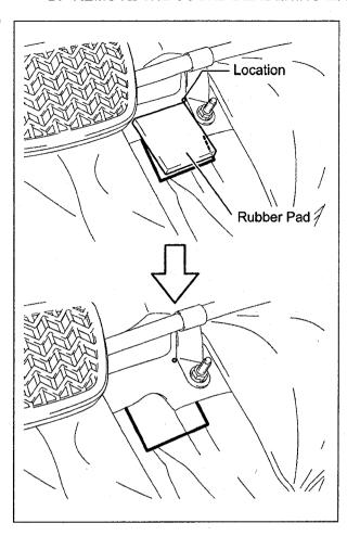
Temporarily place the rubber pad on the floor panel as shown, and outline the pad on the sound deadening material with a ball point pen.
