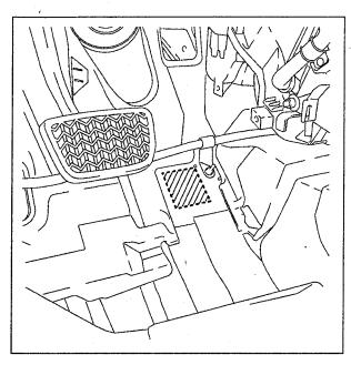
b) Clean and degrease the rubber pad application area.
