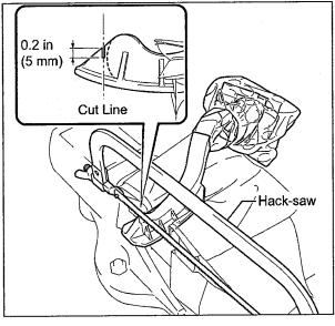
b) Using a hack-saw and cut the pedal 0.2 in (5 mm) to create a guide cut for the reciprocating-saw.
