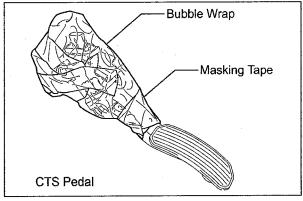
h) While still inside the vehicle, use bubble wrap and masking tape to cover and protect the sensor.
