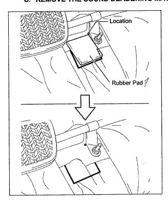
1. Temporarily place the rubber pad on the floor panel as shown, and outline the pad on the sound deadening material with a ball point pen.
