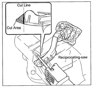
Using a reciprocating-saw and cut off the lower section of the pedal as illustrated.
