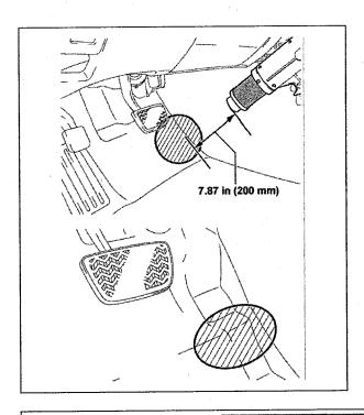
g) Heat the floor carpet area for 2 minutes as shown and smooth it out by pushing it with your hand. Heat the same area again for another minute, and smooth the carpet firmly.
