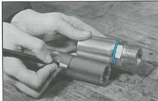
Step 4 Cut hose square using FT1258 bench-mounted cut off tool. Using the bottom edge of the fitting part number as a reference for the length of hose to be inserted into the socket, mark the hose with a china marker to indicate the insertion length.
