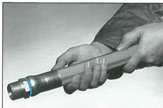
Step 10 Inspect the hose assembly to ensure: • that there is no hose movement in the fitting. • the insertion mark on the hose (from step 4) is still located at the bottom of the socket. The hose assembly is now complete and ready for service (see In Service Inspection below).
