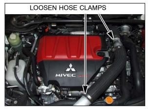
2. Remove the air intake hose by loosening the hose clamps.
