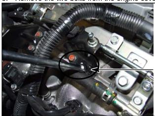
REMOVE ENGINE COVER BRACKET (2 BOLTS)
