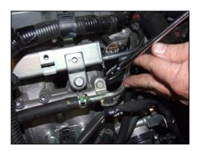
7. Remove the bolt for the vacuum pipe located in front of the engine. Retain this bolt.
